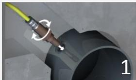
1. Remove stopper from exhaust and screw in the lambda sensor
