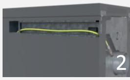
2. Thread the lambda sensor cable through cable track and connect to the print board
