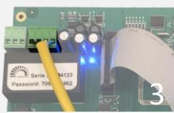
3. Connect cable under O2 Sensor on the V13 print board. The ports are labeled according to the corresponding wire color.
